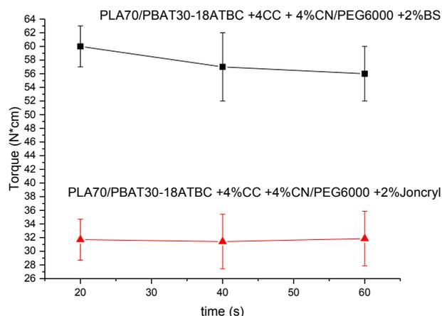
**Figure 2.** Torque data recorded as a function of time during extrusion of plasticized PLA/PBAT blends containing CC and CN with BS (squares) or Joncryl (triangles)
